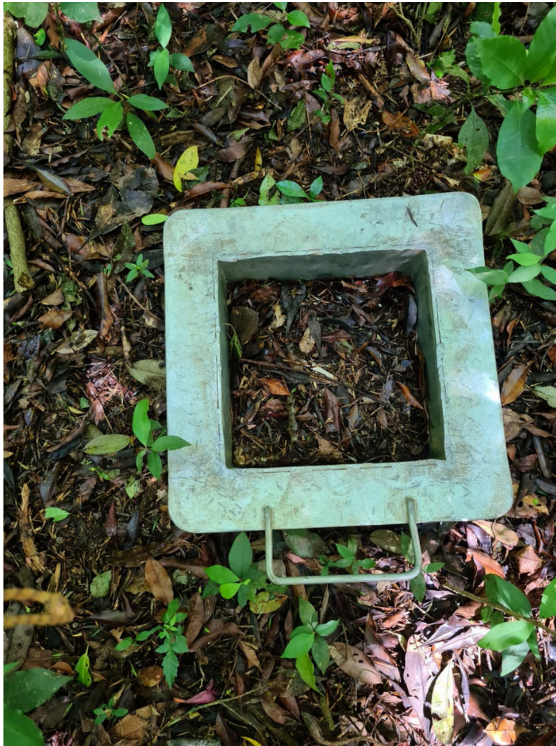
Figure 6. Metal template for collecting soil macrofauna up to 10 cm depth using the TSBF method. Photo: George Brown.
