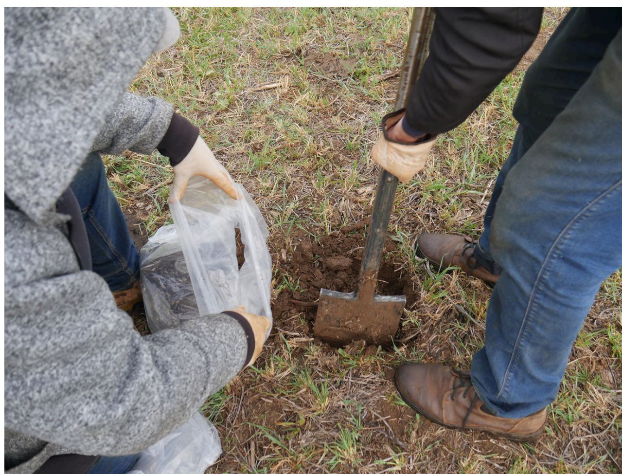
Figure 7. Collection of the monolith without trench excavation. Photo: Marie Bartz.
